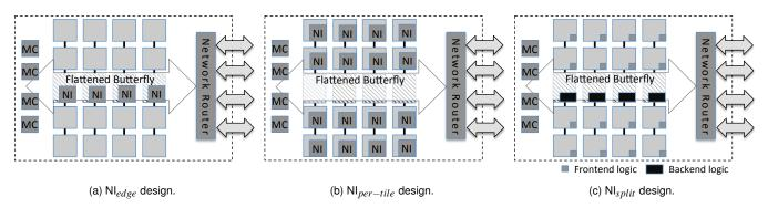
Figure 8: NI design space for NOC-Out-based manycore CMPs. Striped rectangles represent LLC tiles.
