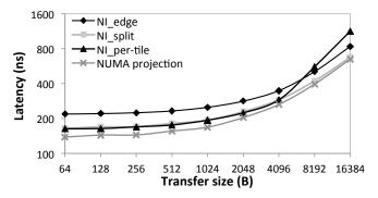
Figure 9: Latency for synchronous remote reads on NOC-Out.
