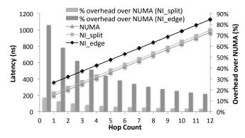
Figure 5: Projection of the end-to-end latency of a cache-block remote read operation for multiple intra-rack network hops. Bars map to the right y-axis, lines to the left y-axis.
