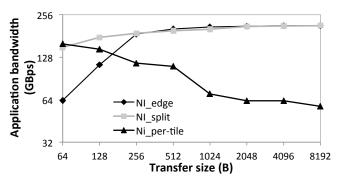
Figure 7: Application bandwidth for async remote reads.
