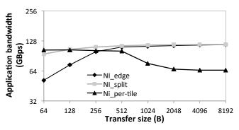
Figure 10: Application bandwidth for asynchronous remote reads on NOC-Out.
