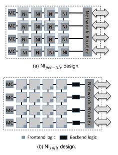
Figure 3: NI design space for manycore chips.
