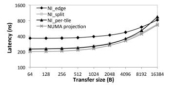
Figure 6: End-to-end latency for synchronous remote reads.
